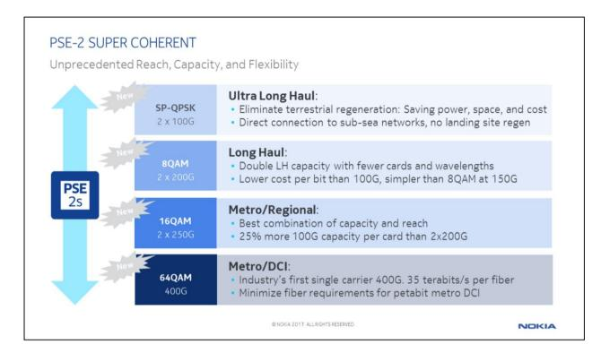
PSE-2 Super Coherent (PSE-2s) increases transport wavelength capacity, distance, and efficiency. It can be programmed to support optimal 100G to 500G transport wavelength capacities and distances for applications ranging from campus to ultra-long haul.
